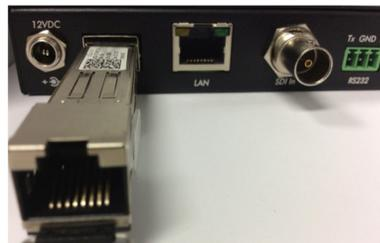
2. Position the SFP Module in front of the SFP socket
