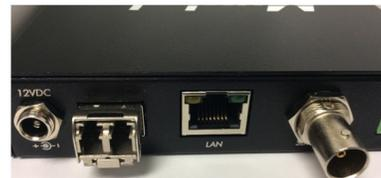
3. Insert the SFP into the slot and ensure is seated properly
