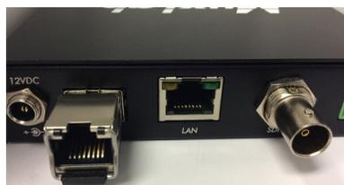
3. Insert the SFP into the slot and ensure is seated properly
