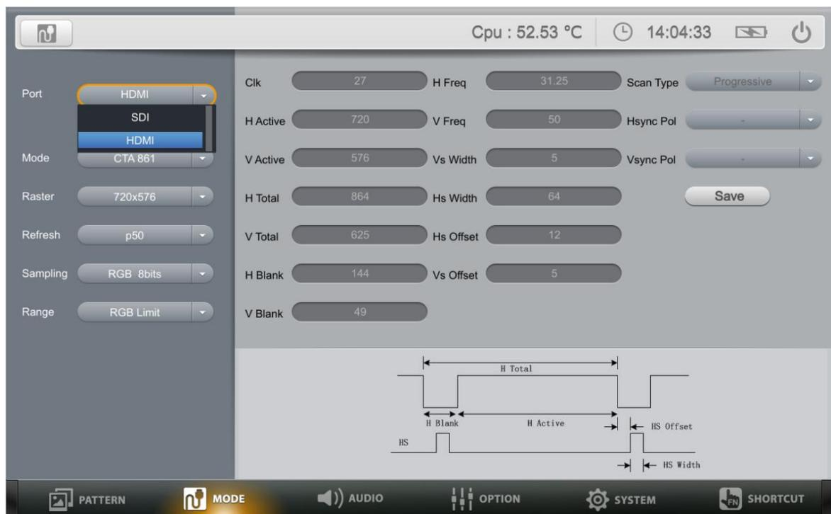
Mode interface supports switch the timing of output signal by using the keys or the mouse. And the related information of the signal output currently can be
