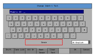
When editing text, the keyboard above is displayed to allow easy editing. Move the cursor to select the key to use and then press  $\mathbf{Ok}$  to press it. The  $\mathbf{Shift}$  menu key causes the keyboard to change to shift mode for the next key.
